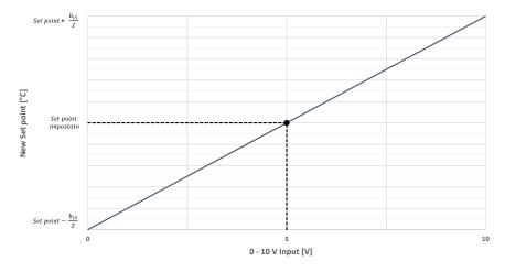
The signal must be applied to terminals X-22.1 and X-22.2- (see wiring diagrams).
