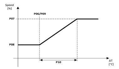
The circulator is at maximum speed in DHW production.
