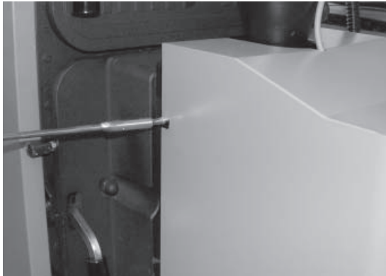
Fig. 13.26: Assembly of burner cover
