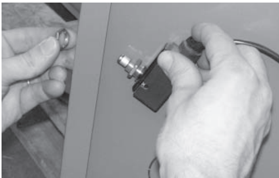
Fig. 13.9: Assembly of microswitch
