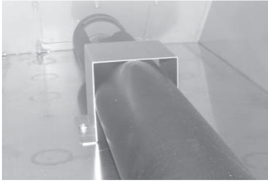
Fig. 13.21: Insertion of the volute into the pellet container
