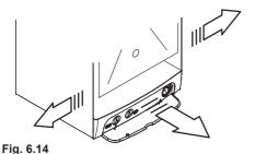
Loosen the screws L and remove the service panel (Fig. 6.15).
