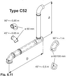
In the last section, the fumes are expelled through a vertical section.
