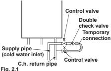
· Open the valves of the filling loop and watch the gauge until it reaches normal filling pressure as shown in Fig. 2.2.
